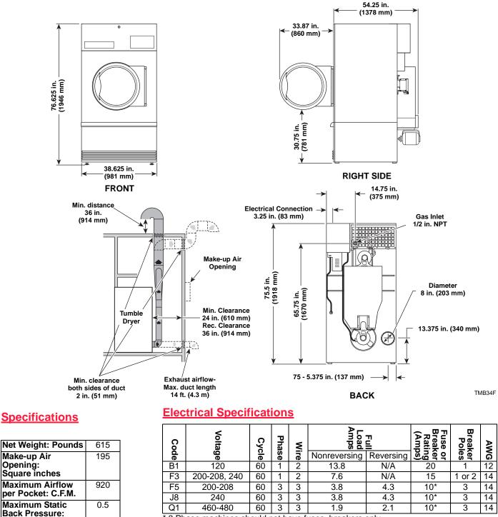
\* 3 Phase machines should not have fuses, breakers only.
